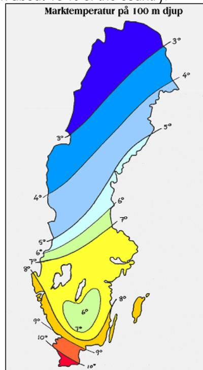
**Swedish ground temperatures at 100 m depth (°C)**
