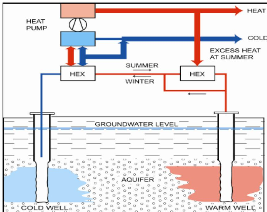
**Figure 1 - The most common ATES configuration**
