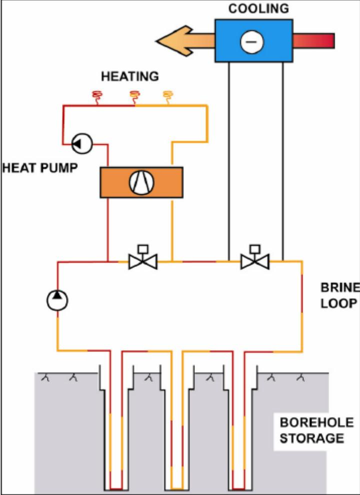
**Figure 2 - The most common BTES configuration in Europe**
