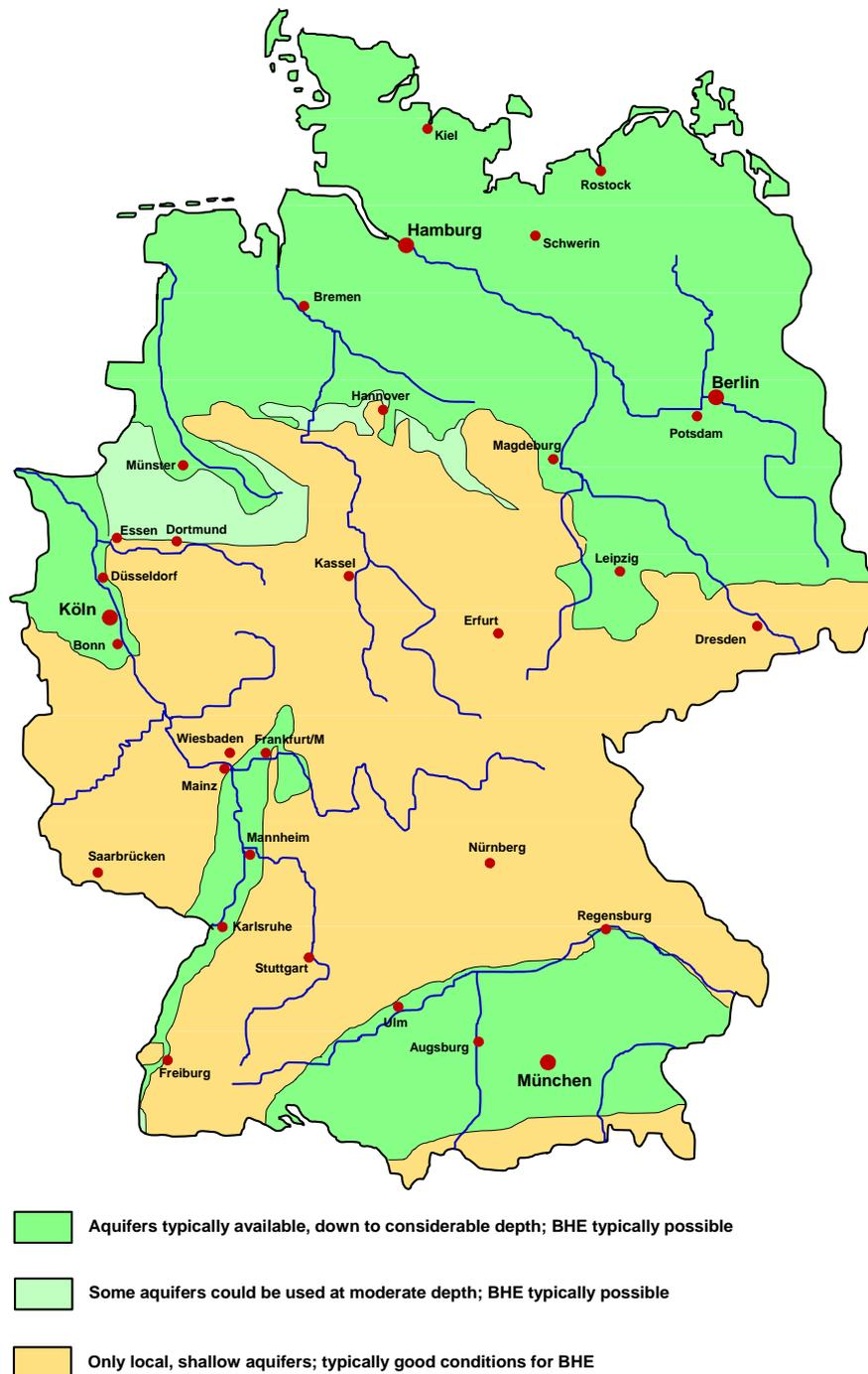
**Figure 6** – Main areas in Germany suited for aquifer storage and BHE; deep geothermal (hydrogeothermal) potential can be found in the green areas only
