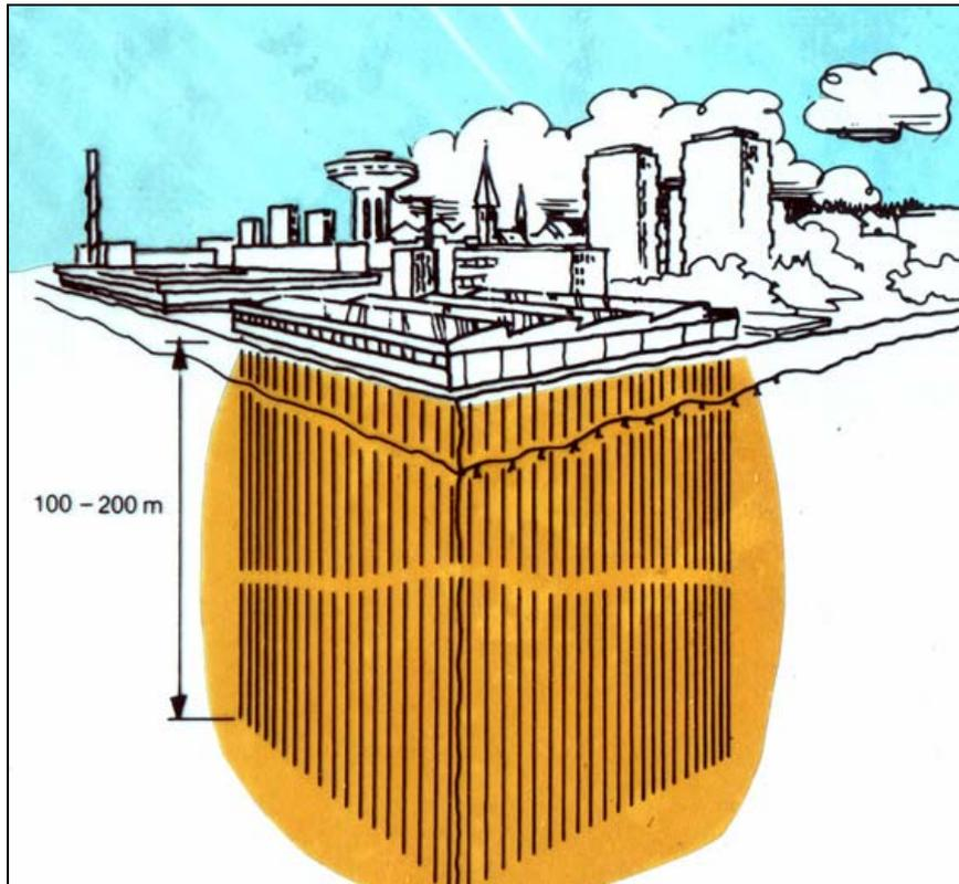
**Figure 3 - The principal for HT BTES systems, in this case with storage of solar energy.**
