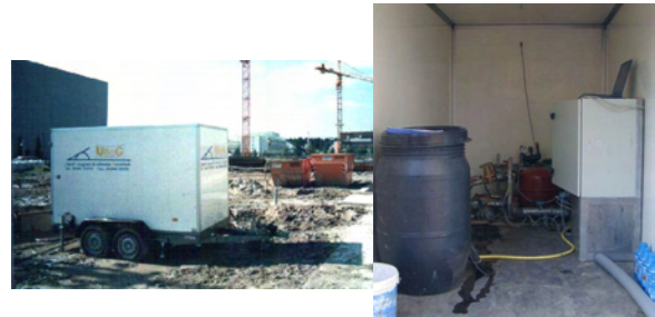
Figure 1: The first UBeG response test rig, as used on the DFS site in Langen in 1999
