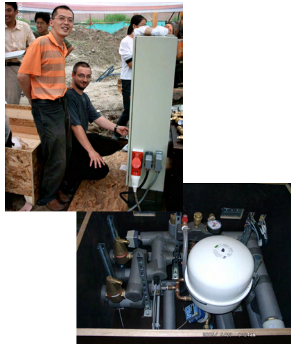
Figure 5: UBeG thermal response test rig exported to China, during training course in Beijing 2004
