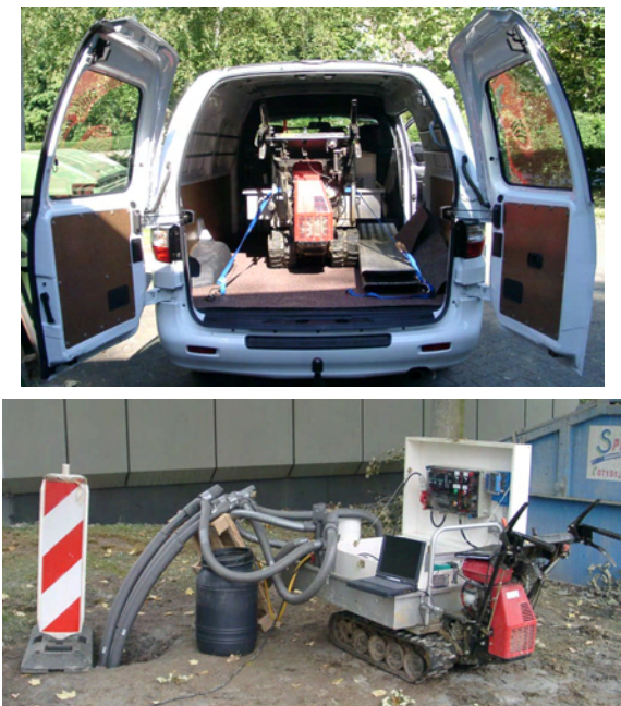
Figure 11: Modern UBeG TRT-equipment, optimized for operation without supervision, and for installation and retrieval by one single person.
