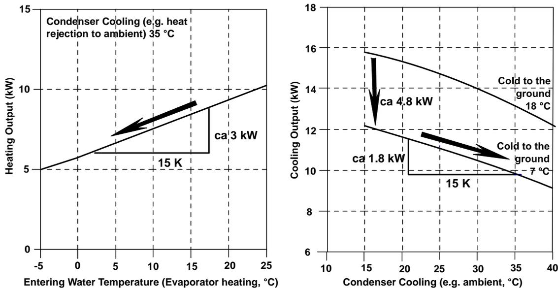
Fig. 2: Substantial drop in heat output with decreasing entering water temperature (left) and drop in cooling output with increasing ambient temperature and decreasing cooling temperature (right); example using heat pump performance data by Alpha-Innotec
