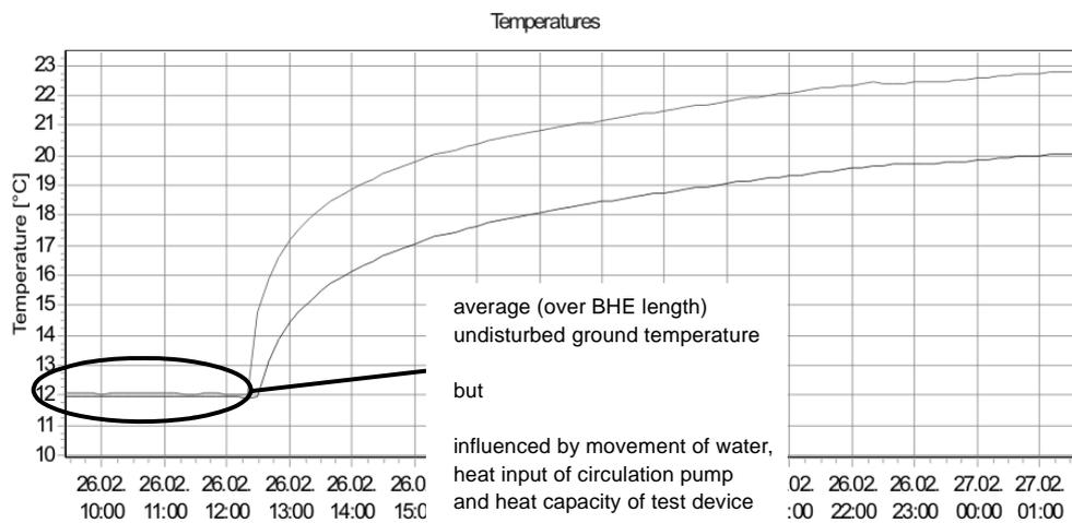
Fig. 4: undisturbed ground temperature from TRT
