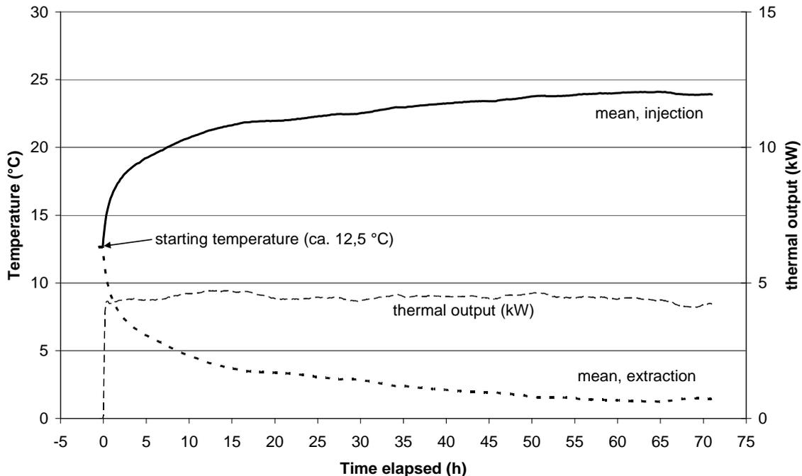
Fig. 1: Measurement principle of TRT (injection example from real field data UBeG); ideal cooling curve (dotted line) would look exactly reciprocal to the heating curve (solid line)
