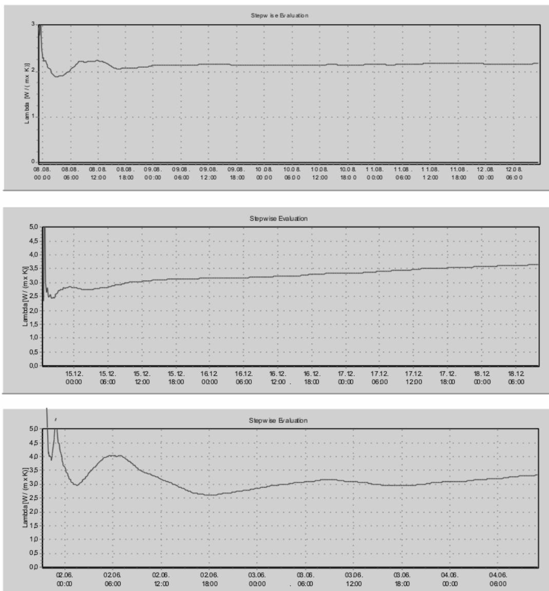
Fig. 3: Examples of stepwise evaluation of TRT: Dominated by conductivity, good reliability (top), dominated by advection and not usable (middle), and high fluctuations and low reliability (bottom)
