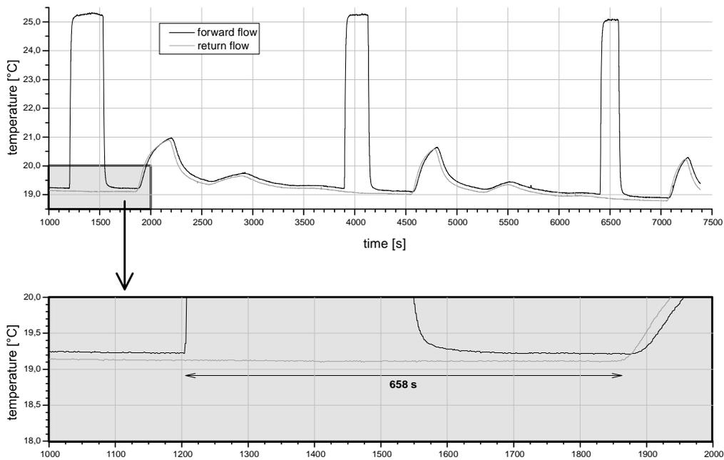
Fig. 8: Principle of Thermo-Impulse method (recurrence of impulse)
