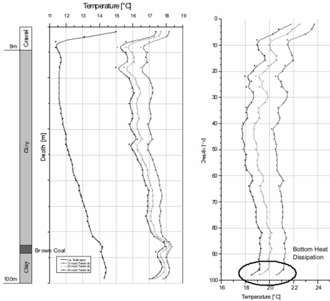
Fig. 7: Features as elucidated by temperature log before and after TRT: presence of a low-conductivity layer (left), prove of final depth (right)
