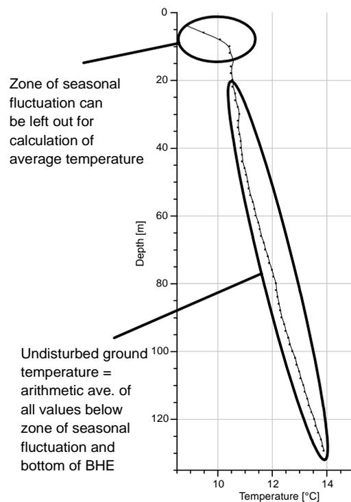
Fig. 5: Temperature profile before performing TRT
