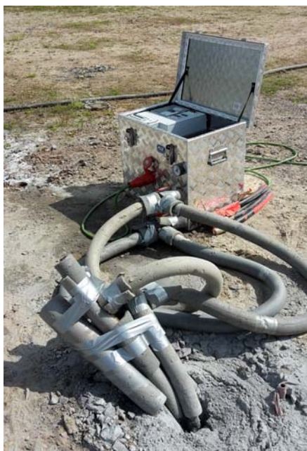
Figure 2: Very mobile TRT on site in Northern Germany in 2016 (devised and built by UBeG; photo Kahl)
