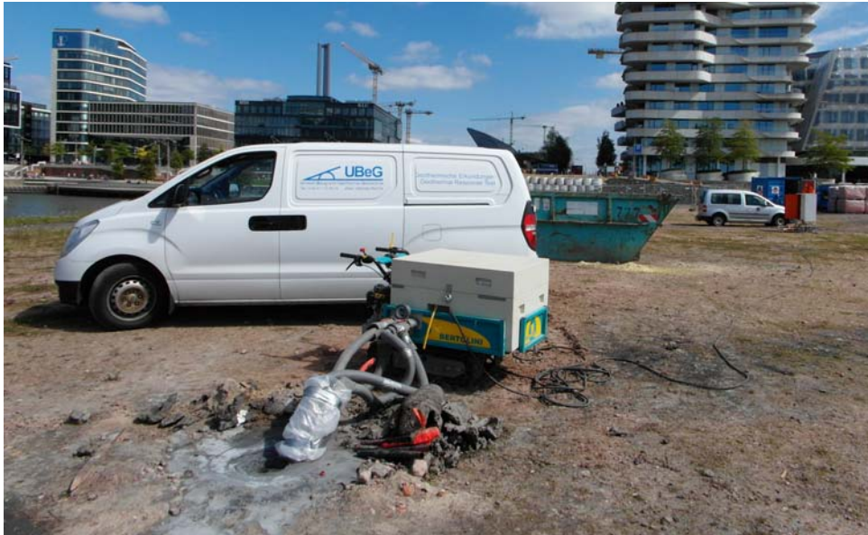
Figure 5: Typical TRT-setup at BHE on a site under development, in summer 2016 (photo Kahl)
