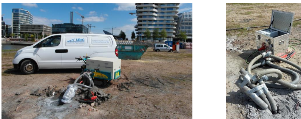
Fig. 8. Typical TRT-setup at BHE on a site under development, in summer 2016 (left) and very mobile TRT on the same site in Northern Germany (right), photos Kahl/UBeG
