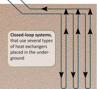
There are several types of closed loops systems, such as: horizontal loops; borehole heat exchangers (BHE); compact forms of ground heat exchangers; thermo-active structures (pipes in any kind of building element in contact with the ground); etc.
